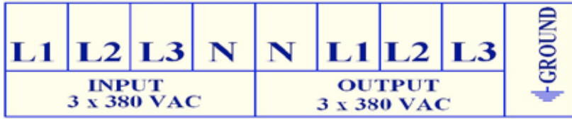
( Figure-2 ) Three-Phase Static Voltage Regulator connection scheme
